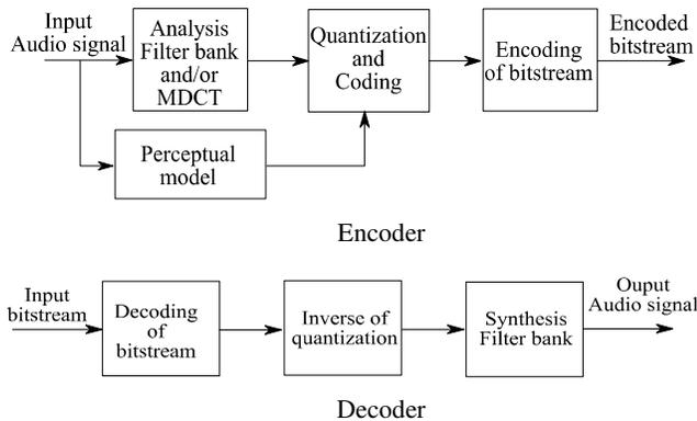
Fig. 1. Basic structure of perceptual encoder and decoder
