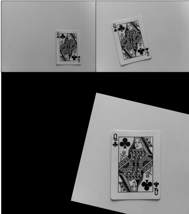
Fig. 6. (Clockwise from top left) Reference image, target image, and registered image from the simulated SIFT VSN network.
