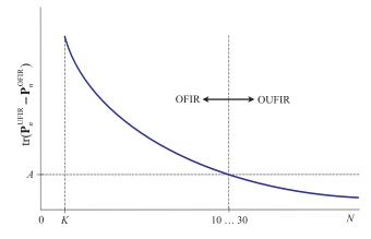
Figure 2: Effect of the estimator window size N on the error difference between the OUFIR and OFIR estimators. Threshold A indicates where the difference becomes visually indistinguishable.
