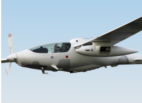
Figure 6. AMBER installed in the under wing pod of the Stemme S15 motor glider during the second test flight in Marnehuizen.
