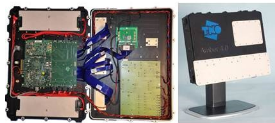
Figure 1. The AMBER radar hardware, including data storage on solid-state disks.
