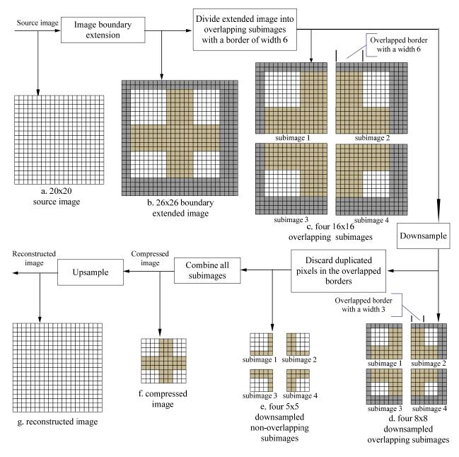
Fig. 3. Illustration of the modified overlap-save subimage method
