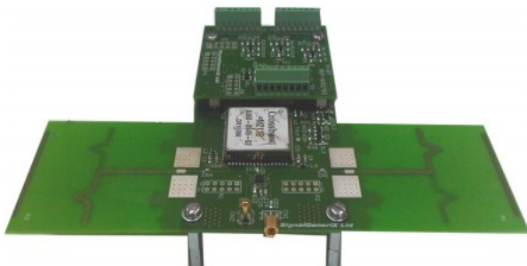
Figure 1: WiseSPOT node with two integrated directional fractal Yagi antennas
