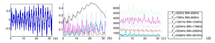
**Fig. 1**. Short-time non-linear analysis of (a) 32 ms of speech of phoneme /a/ by applying Gabor-ESA with six Mel-spaced, 50% overlapped Gabor filters. (b) Instantaneous amplitudes and (c) Instantaneous Frequencies (time axis in milliseconds) (d) Quantities  $F_c$  and BW denote the central frequencies and bandwidths of the Gabor filterbank, both in Hz.
