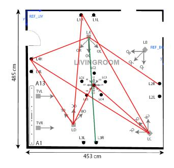
**Fig. 2.** Simulation map of an apartment living room. Green (dashed) and red (solid) lines correspond to the sourcemicrophone location pairs which were simulated in the reverb1 and reverbR sets, respectively.
