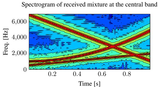
**Fig. 4.** Received signal mixture is comprised of three chirps.
