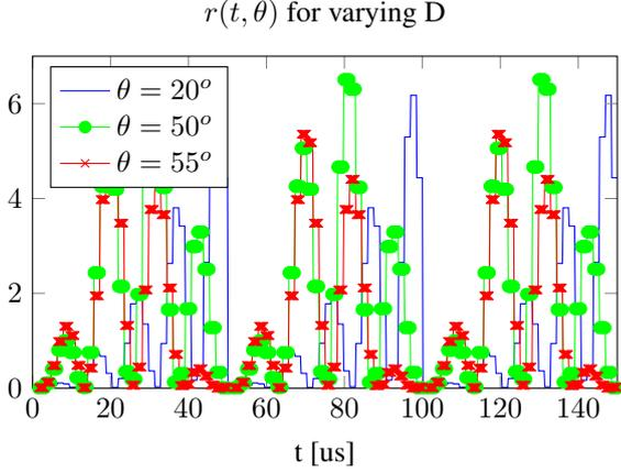
**Fig. 2.** Spatial signature obtained for signals arriving from three different angles. The length of the dipole element is time varying according to (3).
