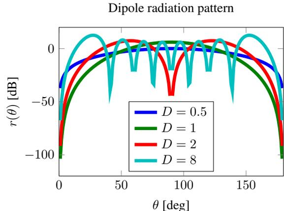
**Fig. 1.** Dipole antenna response for several choices of element length  $D$ .
