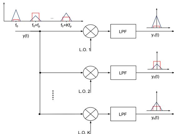
**Fig. 3.** Schematics of demodulating the different bands to baseband, resulting in  $\{y_k(t)\}$  of (6).
