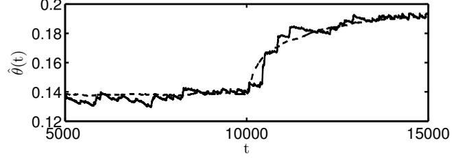
**Fig. 1.** Typical (solid line) and averaged (dashed line) response of the one degree of freedom scheme to a step change of  $\kappa$ .
