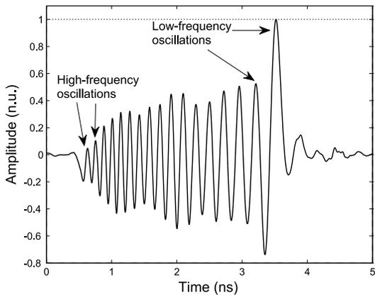
Fig. 3. Measured chirped impulse.
