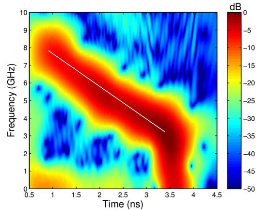
Fig. 5. Spectrogram of the chirped impulse.
