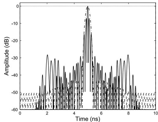
Fig. 6. Compressed pulse for the chirp (continuous line) and ideal Hamming-weighted compressed pulse (dashed line).
