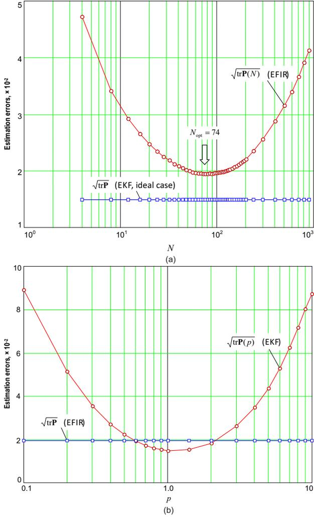
Figure 2: Errors of EKF and EFIR filtering corresponding to Fig. 1: (a)  $\sqrt{\text{tr}\mathbf{P}(N)}$  of EFIR filter and  $\sqrt{\text{tr}\mathbf{P}}$  of EKF and (b)  $\sqrt{\text{tr}\mathbf{P}(p)}$  of EFIR filter and  $\sqrt{\text{tr}\mathbf{P}(p)}$  of EKF.
