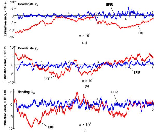
Figure 3: Typical time-domain errors of EKF and EFIR filtering corresponding to Fig. 1 for  $p = 5$  and  $N_{\text{opt}} = 74$ : (a) coordinate  $x$ , (b) coordinate  $y$ , and (c) heading  $\Phi$ .
