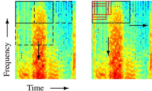
**Fig. 1.** Spectral detail of the clean utterance /t a sh e/. Left hand side: Extraction of frequency bands with time overlap of 10 patches. Right hand side: Extraction of  $12 \times 12$  patches from one frequency band with an overlap of 10 in time and frequency.
