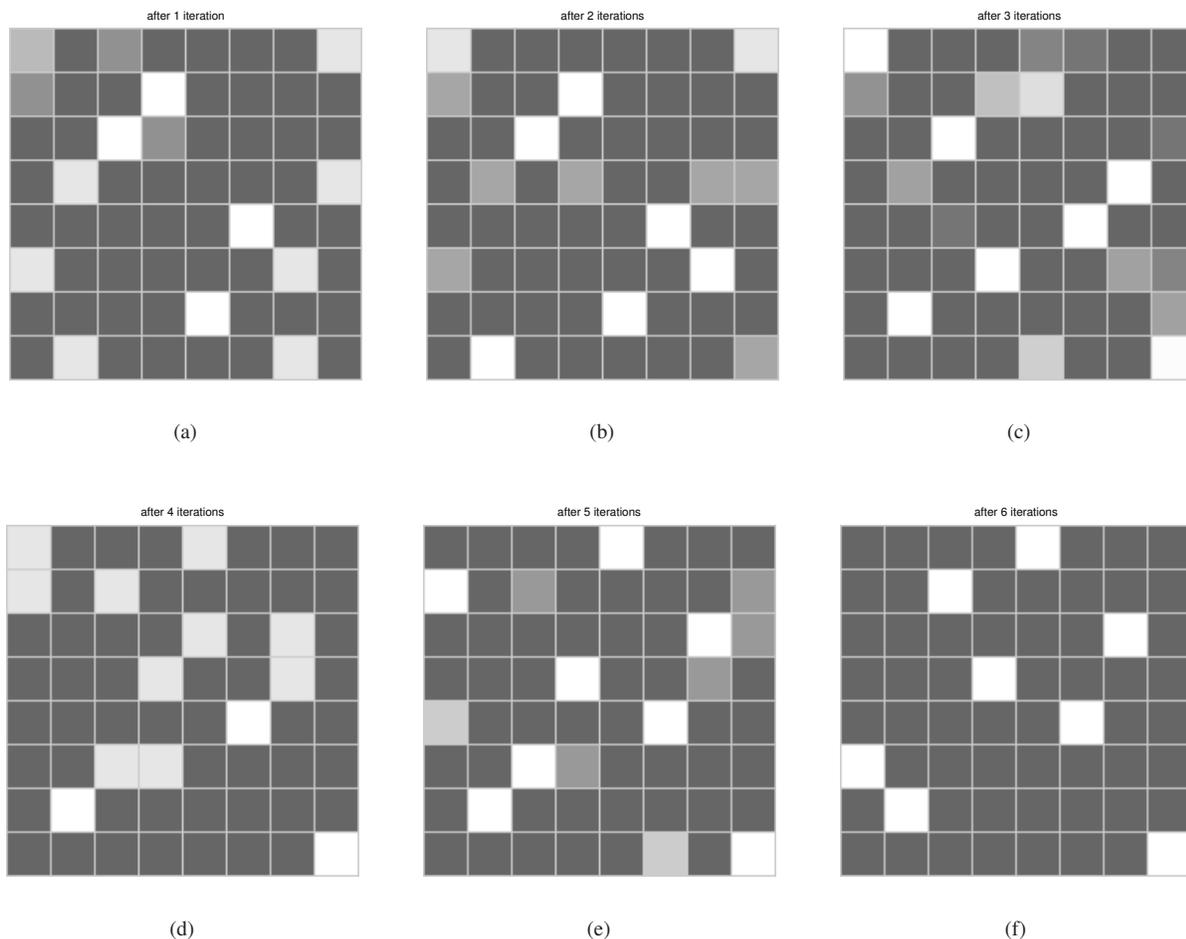
**Fig. 3.** The 2D patterns  $\mathbf{X}^{(k)} = \text{vec}^{-1}(\mathbf{x}^{(k)})$  obtained using the iterative reweighted approach proposed in (14)-(16). The values are shown using grayscale intensity. In this example, the method finds a Costas array after 6 iterations.
