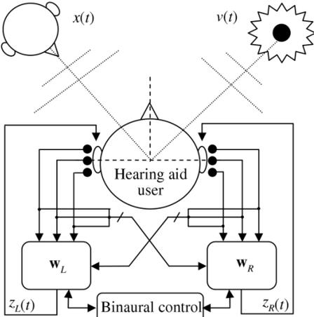
Fig. 1. Binaural system setup.
