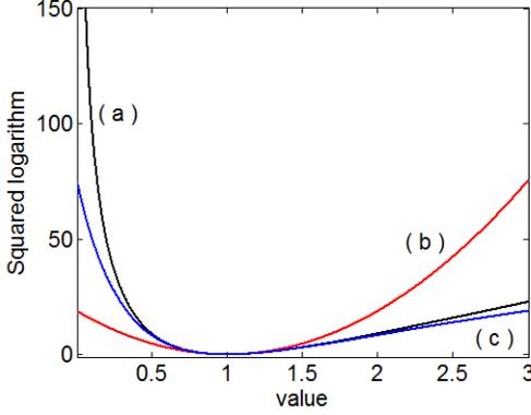
**Fig. 2.** Squared logarithm (a) and approximation by first order Taylor series (b), and first order hyperbolic tangent approximation (c).
