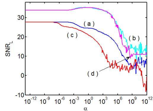
**Fig. 8.** SNR in the left ear. Proposed technique: (a)  $S_0N_{-60}$ , (b)  $S_0N_{60}$ . Technique proposed in [4]: (c)  $S_0N_{-60}$ , (d)  $S_0N_{60}$ .
