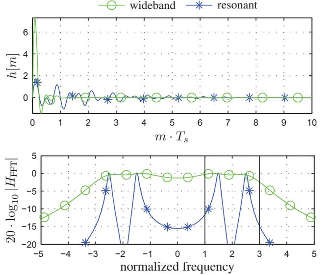
**Fig. 1.** Impulse response (top) and frequency response magnitude (bottom) of simple example systems. The resonant system has  $K=4$  conjugate complex poles  $s_k = \{-0.5 \pm j2\pi 1.5, -0.5 \pm j2\pi 2.5\}$  with  $R_k = \{\mp j0.5, \mp j0.5\}$ . The wideband system has  $K=4$  conjugate complex poles  $s_k = \{-5 \pm j2\pi 1.5, -5 \pm j2\pi 2.5\}$  with  $R_k = \{\mp j2.5, \mp j4\}$ .  $f_u$  and  $f_l$  are indicated by two solid black vertical lines.
