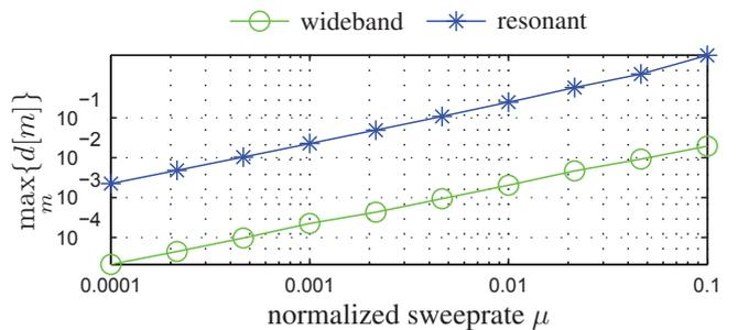
**Fig. 4.** Maximum of error  $\max_m\{d[m]\}$  versus sweep-rate for both, resonant and wideband systems. The error in the wideband system is approximately one percent of the error obtained for the resonant system. For both systems, the error linearly scales down with the sweep-rate.
