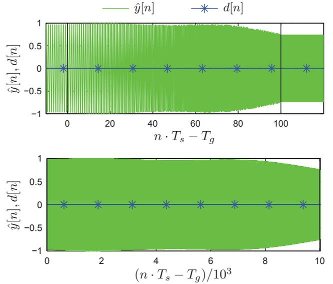
**Fig. 3.** Quasi-Stationary responses and distortion signals obtained for LFM CW excitation with sweep-rates of (top)  $\mu = 0.02$  and (bottom)  $\mu = 0.0002$  applied to wideband example system. The distortion component is small for both  $\mu$ .
