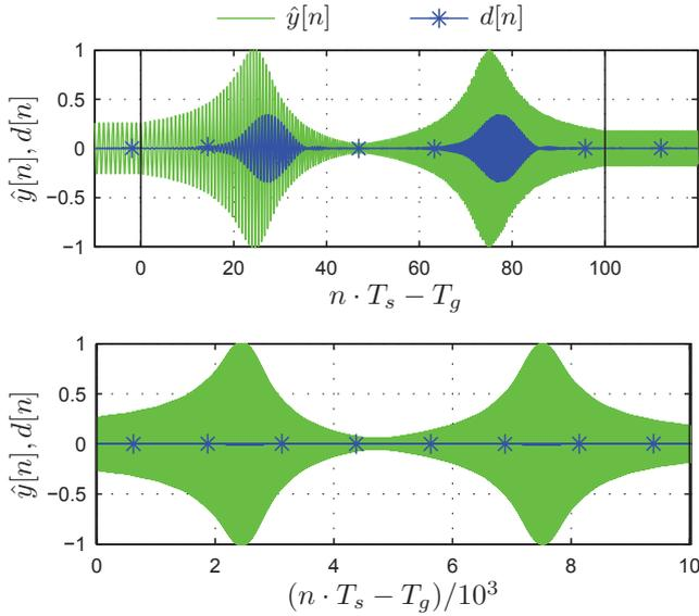
**Fig. 2.** Quasi-Stationary responses and distortion signals obtained for LFM CW excitation with (top)  $\mu = 0.02$  and (bottom)  $\mu = 0.0002$  applied to resonant example system. The fast sweep results in a significant distortion component.
