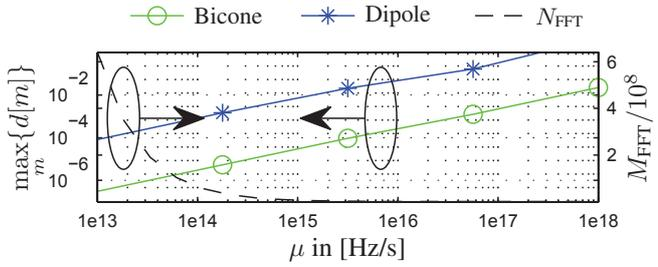
**Fig. 6.** Error maximum  $\max_m \{d[m]\}$  and FFT length  $M_{\text{FFT}}$  vs. sweeprate for both, Bicone and Dipole. For both systems, the error linearly scales down with the sweeprate.
