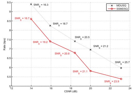
Fig. 5. CSNR vs rate plot,  $SNR_g$  values for each point are reported in dB.
