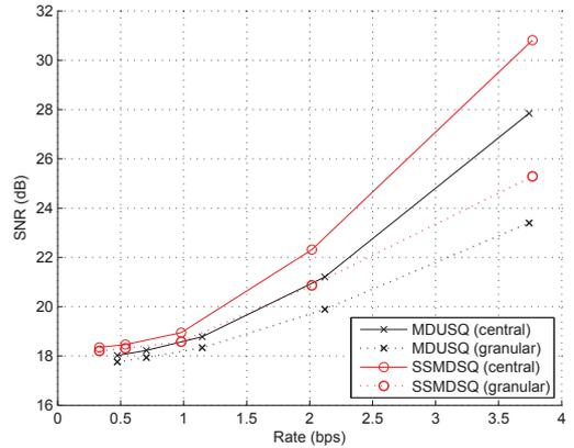
Fig. 4. RD comparison between MDUSQ and SSMSDSQ. SNR of the central reconstruction and Granular SNR are plotted vs the total bitrate. The Granular SNR is computed as:  $SNR_g = 10 \cdot \log_{10}(\sigma_X^2 / \sqrt{D_c D_s})$ , with  $D_c$  and  $D_s$  being the central and average side MSE distortions, respectively.
