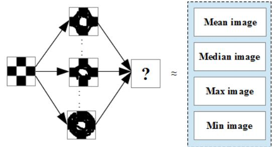
**Fig. 4.** Random pattern changes during P&S process.
