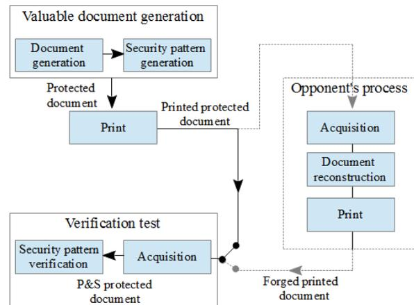
Fig. 1. General verification system for document protection.
