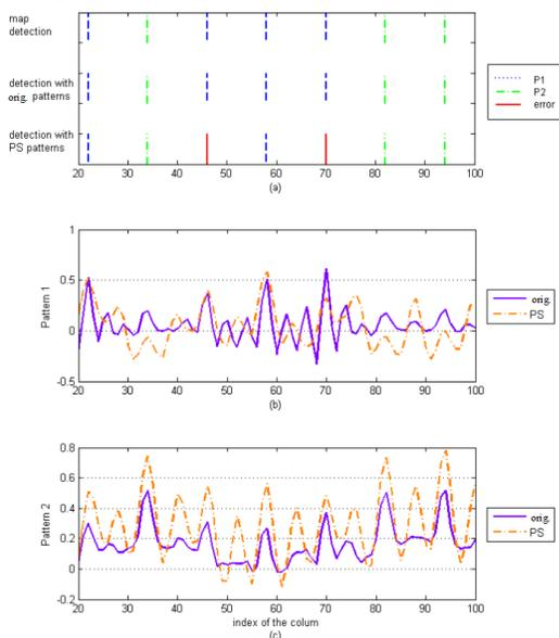
**Fig. 11.** Correlation values of one line of textured image for pixels in interval  $[20 \dots 100]$ .
