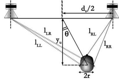
**Fig. 2.** Geometrical representation of the stereophonic reproduction environment using two loudspeakers.
