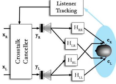
**Fig. 1.** A block diagram of an audio system that can adjust the sweet spot with relation to the listener position.
