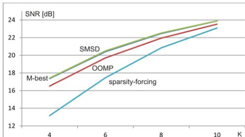
**Fig.4.** SNR for LD-CELP coder with signal model (3) - confidence interval for all SNR values: 0.05 dB
