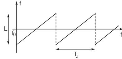
Fig. 1. Frequency sweep of the chirp jamming signal.
