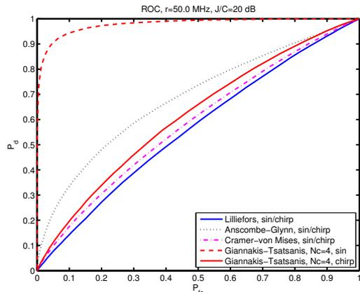
**Fig. 2.** ROC curves for Anscombe-Glynn, Lilliefors, Cramér-von Mises and Giannakis-Tsatsanis tests with sinusoidal and chirp interference signals.
