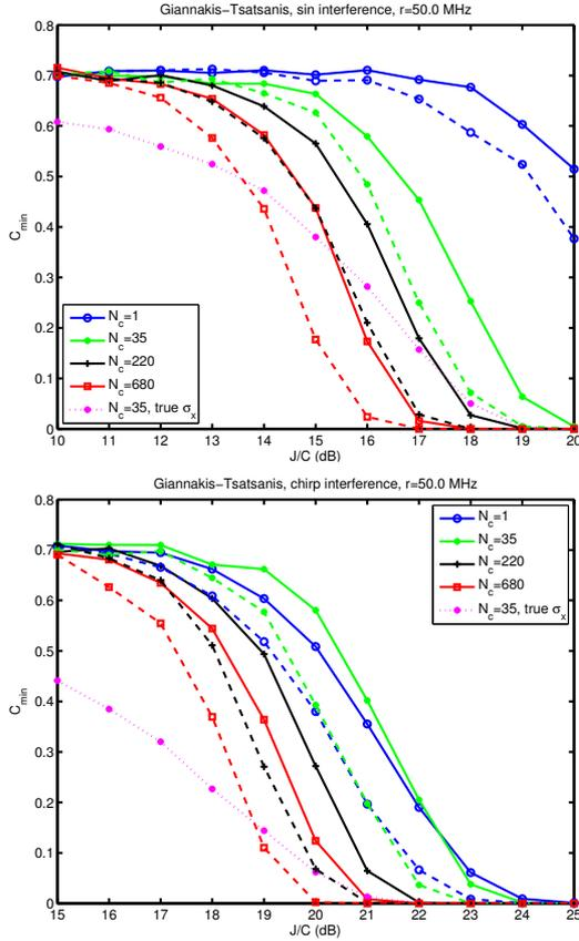
Fig. 3. ROC metrics  $C_{\min}$  for the G-T test with sinusoidal (top) and chirp (bottom) interference.
