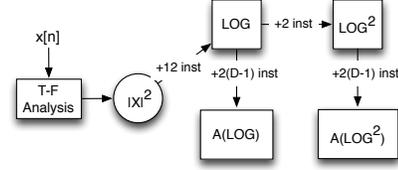
**Fig. 2:** Number of instructions associated to the computation of the proposed features.
