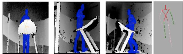
**Fig. 4.** Human Skeleton from 3 different angles with occlusion, and the resulting skeleton, using joints from proper sensors.
