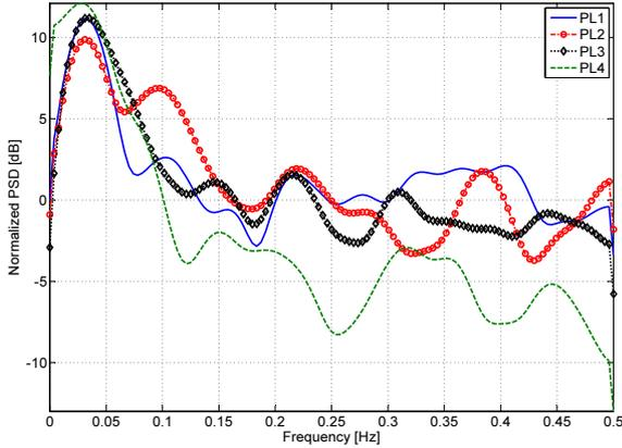
**Fig. 2.** PSDs of  $C/N_0$  measurements (after DC removal) from four pseudolites placed in the corners of a large meeting room. The user circled around the large table placed in the middle of the room.
