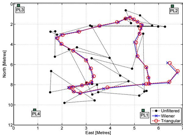
**Fig. 6.** Comparison between the navigation solutions obtained using the Wiener and triangular filters used for smoothing  $C/N_0$  measurements. The navigation solution obtained using unfiltered measurements is also provided as a term of comparison. Loop performed in a large meeting room.
