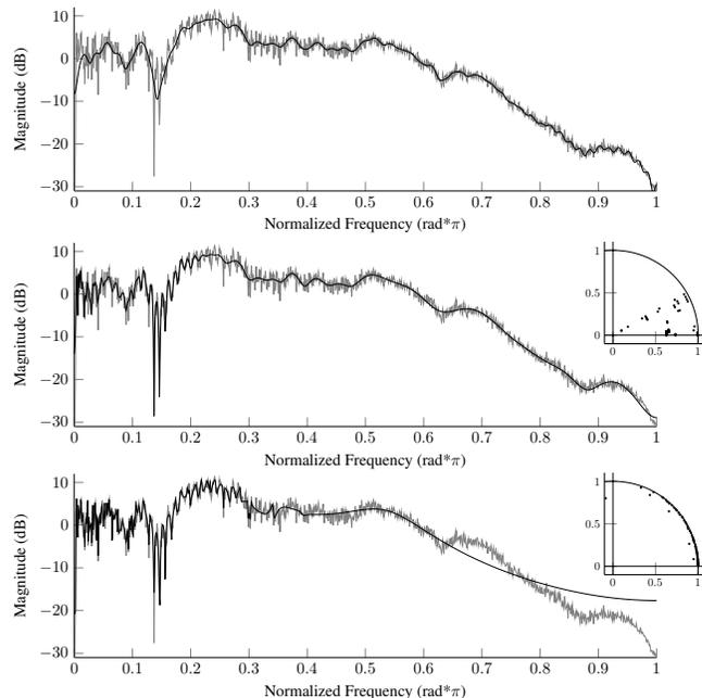
**Fig. 4:** Estimated magnitude response for the all-zero model (top), for the OBF model with the proposed method (middle) and with the BU method (bottom), together with the selected pole set ( $\mu = 0.04$ ,  $n_\theta = 122$ ). The target response is shown in grey.
