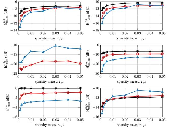
**Fig. 3:** (left) The average NMSE in (6) for the entire response (top) and for the early (middle) and late response (bottom). (right) The average NMSE in (7) for the entire spectrum (top) and for the frequency regions  $[0, \frac{\pi}{6}]$  (middle) and  $[\frac{\pi}{6}, \pi]$  (bottom). For the all-zero model ( $\blackstar$ ) and for the OBF model, calculated with the proposed method ( $\circ$ ) and the BU method ( $\triangle$ ).
