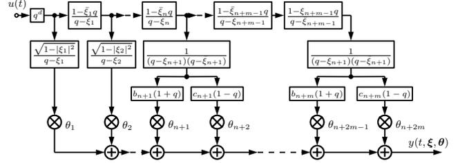
**Fig. 1:** The mixed Kautz model structure, with parameters  $b_i = |1 - \xi_i| \sqrt{1 - |\xi_i|^2} / 2$  and  $c_i = |1 + \xi_i| \sqrt{1 - |\xi_i|^2} / 2$ .
