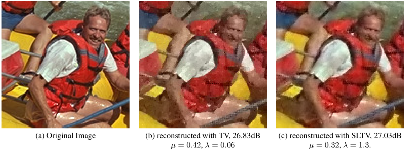
Fig. 1. Joint demosaicing-denoising experiment on image 14 of the Kodak test base. The PSNR values correspond to the whole image, not to the crop selected here. The parameters \mu and \lambda were empirically optimized to maximize the PSNR. 100 iterations of the algorithm were run.
