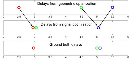
**Fig. 3.** Example of delay disambiguation by a NN approach. Each circle denotes a delay whose value is given by the x-axis. Each ambiguity free delay calculated from geometry is associated to the closest delay estimated from the signals.
