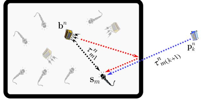
**Fig. 1.** The figure shows the real source  $\mathbf{b}^n$  together with the image source  $\mathbf{p}_k^n$ . The image source is positioned such that the sound path in red equal the blue path coming from  $\mathbf{p}_k^n$
