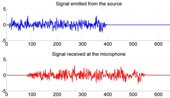
**Fig. 4.** Example of emitted signal from a generic source (left), and related acquired signals at a generic microphone (right).
