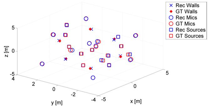
**Fig. 5.** Ground truth and reconstruction of walls, microphones and sources positions yielded by the proposed algorithm.
