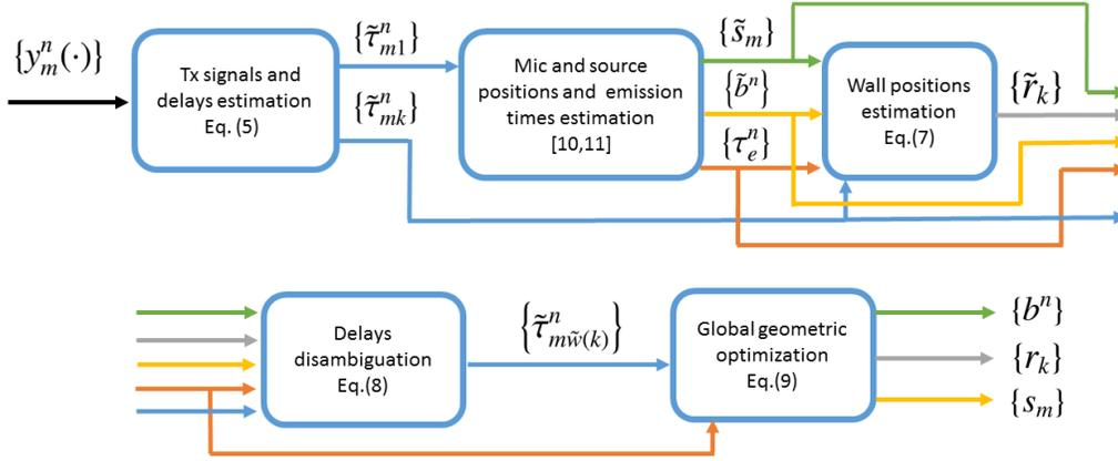
**Fig. 2.** Diagram of the overall method. Each box corresponds to a computational step as implemented by our approach. The figure also presents corresponding input (audio signals) and outputs (mic/sound source position, the transmitted signal, delays and room walls position).
