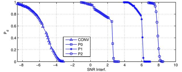
**Fig. 4.** Probability of detection versus SNR for  $P_{fa} = 10^{-3}$ . The scenario considers a BPSK primary signal (rectangular pulse shape, 8 samples per symbol) with SNR = 0dB, located at normalized frequency 0.25. There is a pure tone interference located at normalized frequency 0.75.
