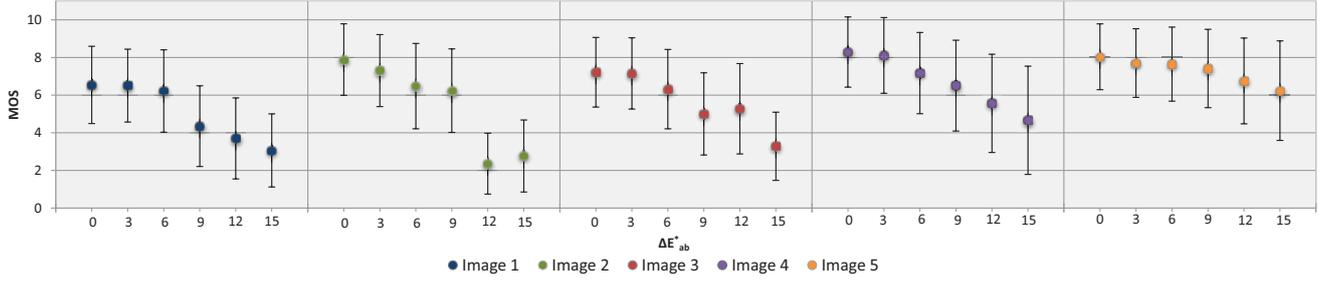
Fig. 1. MOS as function of  $\Delta E_{ab}^*$  for all test images.
