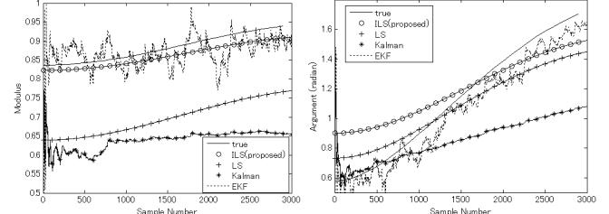
Fig. 2. Estimation of the pole modulus (left) and argument (right) for a 2<sup>nd</sup>-order TVAR process
