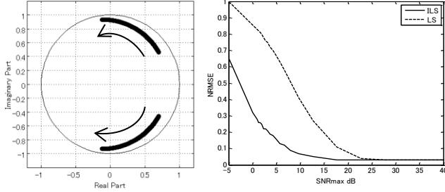
Fig. 1. Evolution of the poles of the AR process in the  $z$ -plane (left) and NRMSE for various  $SNR_{max}$  (right).
