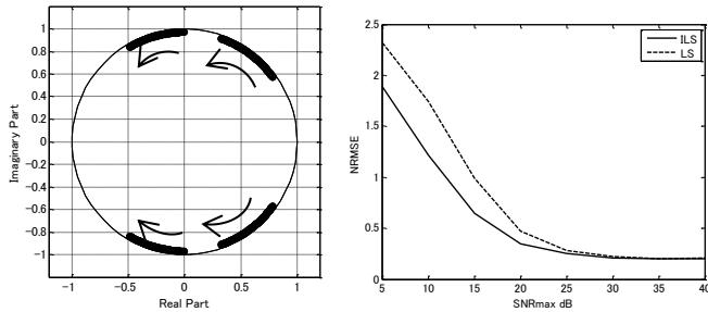
Fig. 4. Evolution of the poles of the AR process in the  $z$ -plane for  $p = 4$  (left) and NRMSE for various SNR (right).
