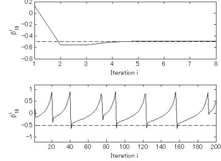
Fig. 3. Convergence features of the weight estimation  $\beta_{10}$  for  $SNR_{max} = 2.7$  (top) and -5.0 dB (bottom), (the break line indicates true value  $\beta_{10} = -0.5$ ).
