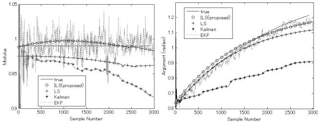
Fig. 5. Estimation of a pole modulus (left) and argument (right) for a 4<sup>th</sup> order TVAR order
