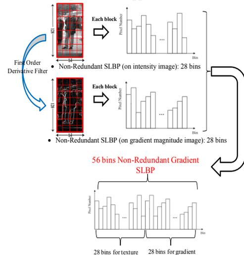
Fig. 6. Non-redundant patterns are calculated on both intensity and gradient magnitude maps
