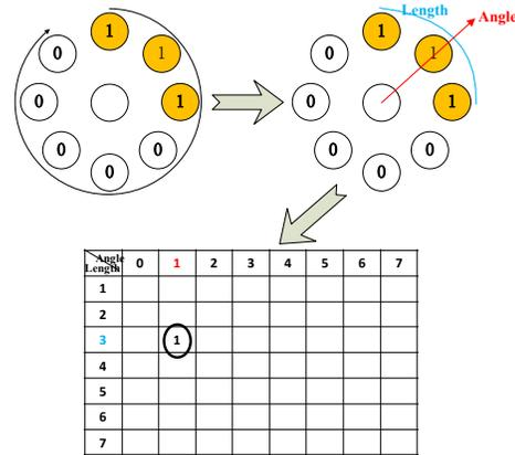
Fig. 2. Feature extraction process of SLBP for each pixel
