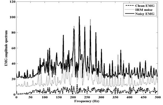
**Fig. 3.** Amplitude spectrum of fMRI noise, EMG signal in normal and fMRI conditions of acquisition. Spectrum are slightly shifted for the sake of clarity.
