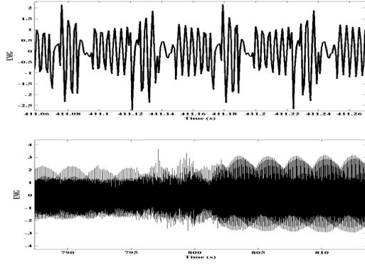
**Fig. 2.** A zoom on fMRI noise to show its harmonicity (a) and its variation over time (b).
