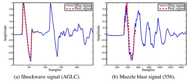
**Fig. 4.** Deconvolving the components of a gunshot signal. The sample rate is 96 kHz.
