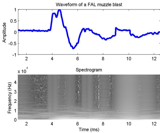
Fig. 8. Spectrogram of the muzzle blast from a FAL, an example of a image from which texture features are selected.
