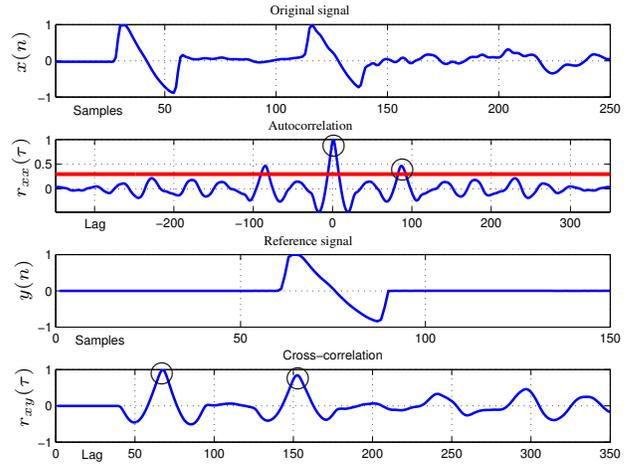
**Fig. 2.** SW signal  $x(n)$  from an AGLC shot: autocorrelation  $r_{xx}(\tau)$  and cross-correlation  $r_{xy}(\tau)$  with a reference signal  $y(n)$ . The sample rate is 96 kHz.
