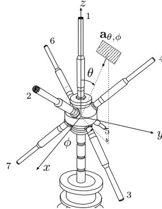
**Fig. 5.** Microphone array and angles of interest.
