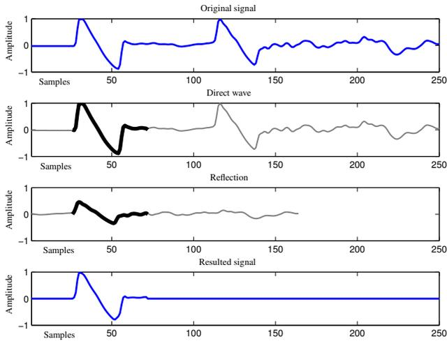
**Fig. 3.** Deconvolving a shockwave using autocorrelation. The sample rate is 96 kHz.
