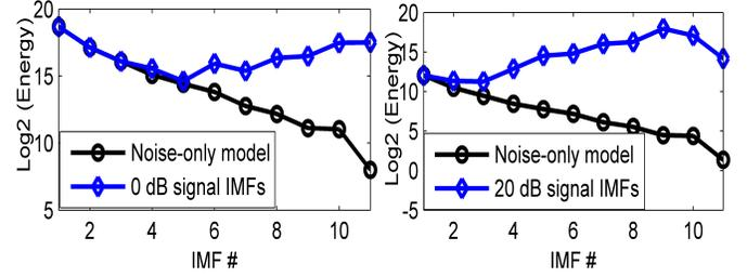
Fig. 5. The WGN model [9] to identify noise free IMFs.
