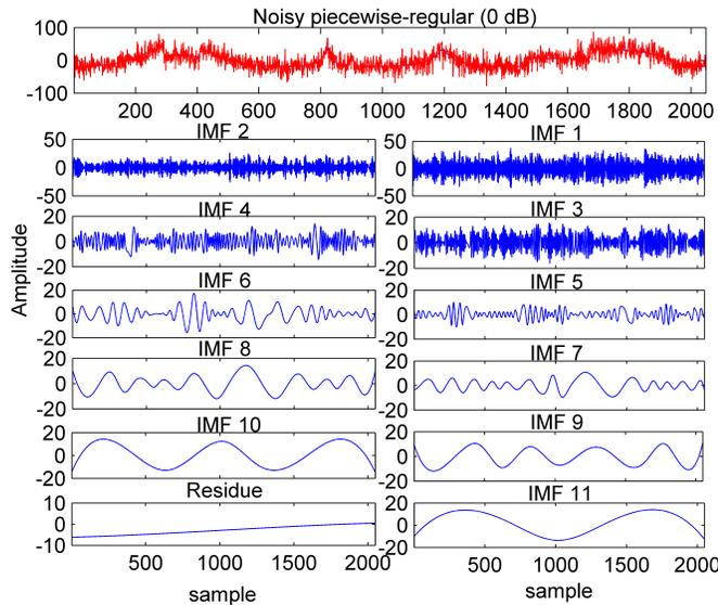
**Fig. 1.** The decomposition of piecewise regular signal with 0 dB SNR.
