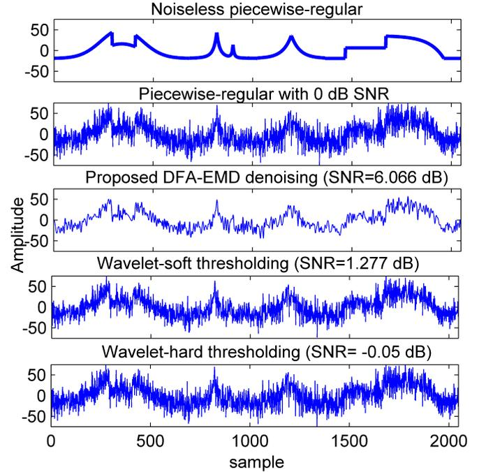
**Fig. 2.** Comparison of the proposed DFA-EMD based denoising at 0 dB SNR.
