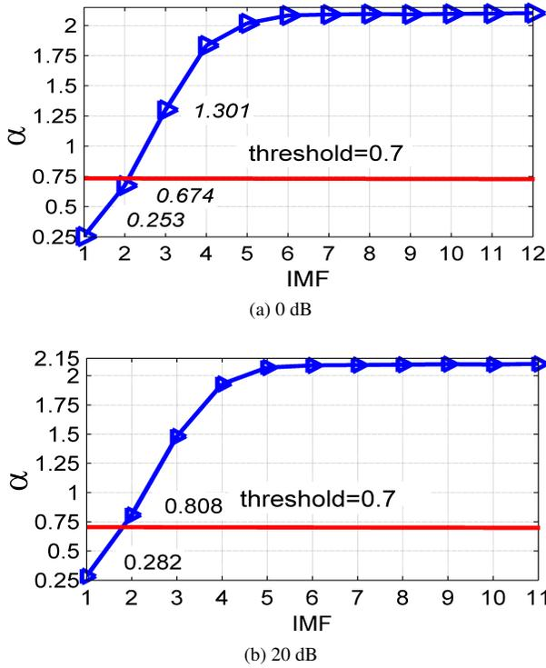
Fig. 4. DFA slopes of the decomposed IMFs for piecewise-regular signal.
