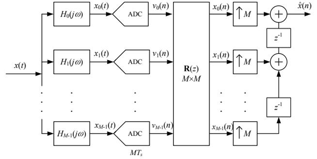
Fig. 2. Generalized structure of the Hybrid Filter Bank.
