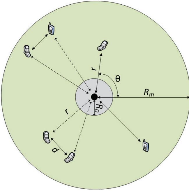
Figure 1. Network diagram showing a network consisting of a macrocell, and D2D communication links. The solid lines represent data traffic path while the dashed lines represent signaling.
