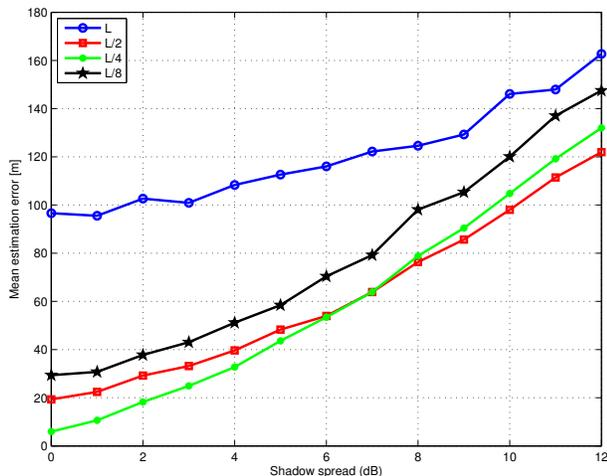
Fig. 7. Performance of maximum approach for different search space sizes
