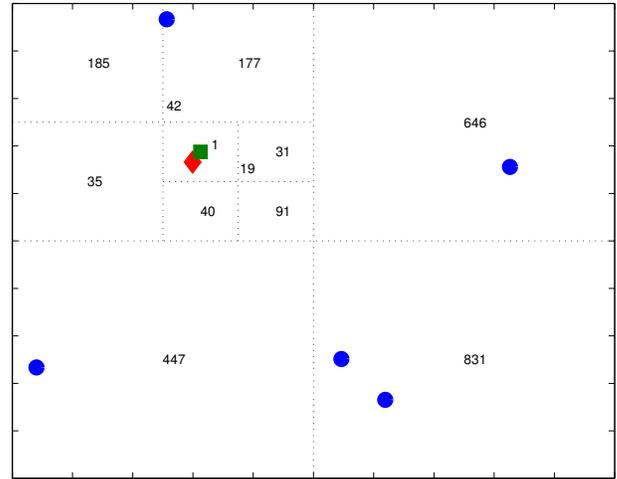
Fig. 2. An example of 3 level 2x2 partitioning for iterative grid search.
