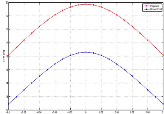
Fig. 4: Optimized SINR as a function of frequency synchronization errors ( $\Delta\nu$ ) ( $CP=32$ ,  $SNR=30dB$ ,  $B_dT_m = 10^{-2}$  and waveform support duration equal to  $3T$ ).
