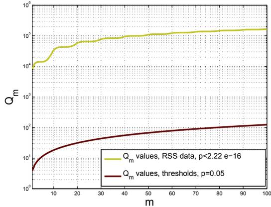
**Fig. 2.** Ljung-Box Q-test statistics obtained for  $m = 1, 2, \dots, 100$  time lags from  $N = 15000$  RSS samples. Threshold values for  $\alpha = 0.05$  are also presented
