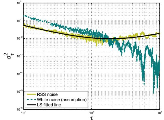
**Fig. 3.** AVAR and LS fitted line for the real RSS dataset.
