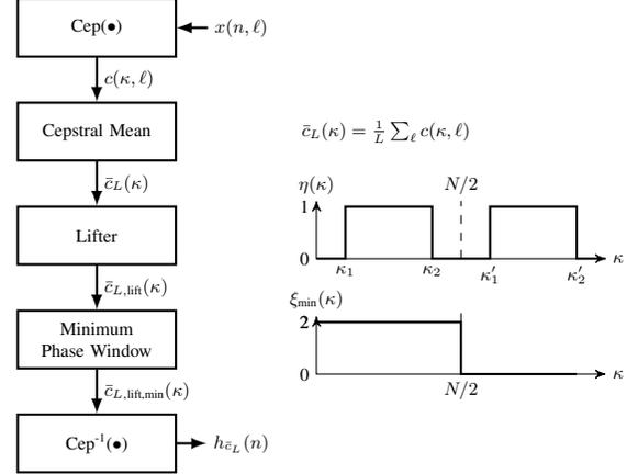
**Fig. 1.** Algorithm to estimate the stationary impulse response within the audio signal.
