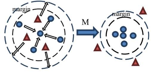
**Fig. 3** Illustration of the distribution of instances belonging to two classes [19]. By applying the metric learning algorithm (minimizing the distances between instances in the same class while keeping instances from the other class far away), the input instance is surrounded by training instances of the same class.
