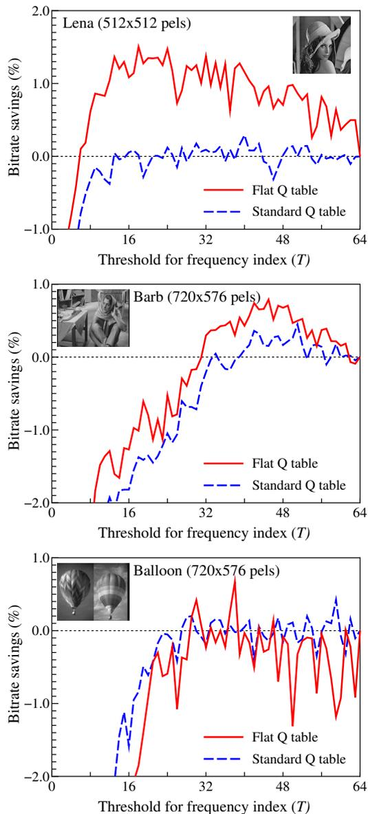
Fig. 6. Bitrate savings over the block-wise intra prediction ( $T = 64$ ).
