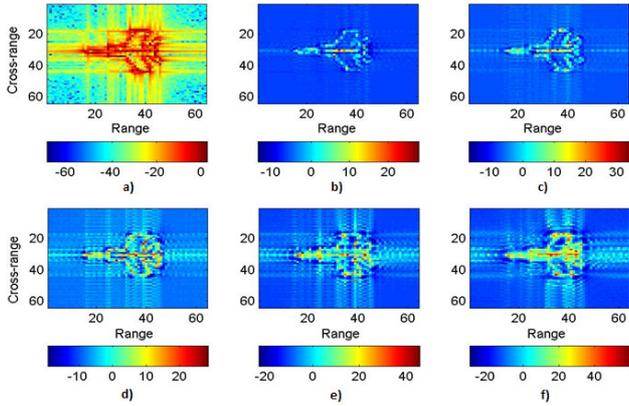
**Figure 2.** Radar images obtained using a) polar-format algorithm and radar images using l2-norm minimization with SVD truncation with modelling level 25 and number of scattering centers b) 30, c) 50, d) 70, e) 90, f) 110
