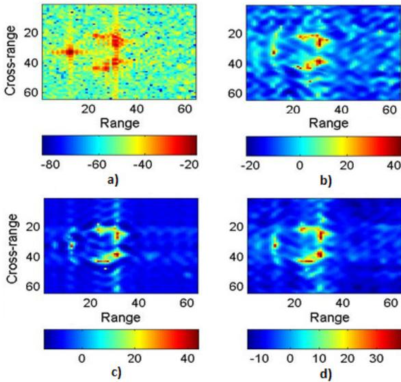
**Figure6.** ISAR images for esairbus data using a) polar format algorithm b) l2-norm minimization, c) l2-norm minimization with SVD truncation (number of scatterers=20), d) l2- norm minimization with l1-norm penalty function with  $\lambda=0.5$  (S/N=10dB, modeling level=10)
