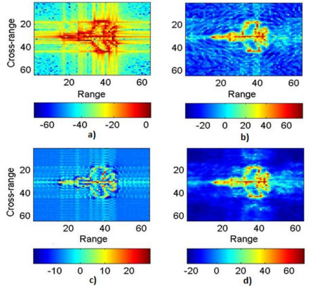
**Figure 1.** ISAR images using a) polar-format algorithm, b) l2 minimization c) l2 minimization with SVD truncation, d) proposed l2 minimization with l1 penalty,  $\lambda=1.0$
