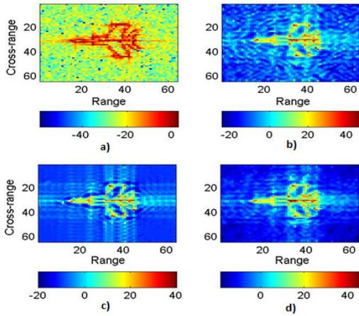
**Figure5.** ISAR images for mig25 data using a) polar format algorithm b) l2-norm minimization (modeling level=20), c) l2-norm minimization with SVD truncation (modeling level=20 and number of scatterers=70), d) l2- norm minimization with l1-norm penalty function (modeling level=20) with  $\lambda=4.0$  (S/N=10dB)
