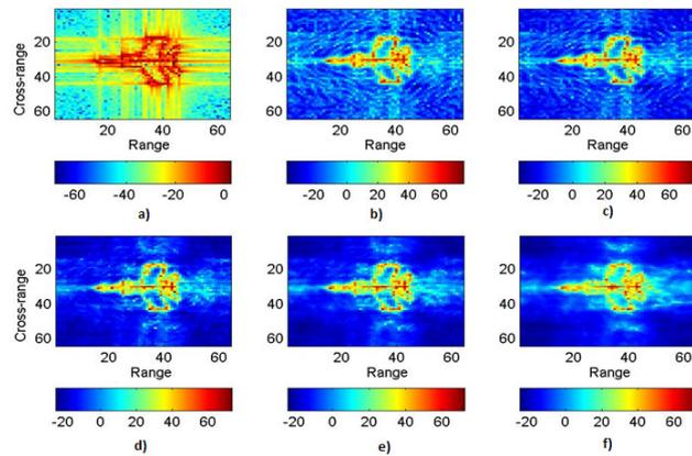
**Figure3.** ISAR images for mig25 data using a) polar-format algorithm, the proposed method with regularization parameters b)  $\lambda = 0.001$ , c)  $\lambda = 0.1$ , d)  $\lambda = 0.5$ , e)  $\lambda = 1$ , f)  $\lambda = 4$
