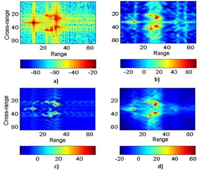
**Figure 4.** ISAR images using a) polar-format algorithm, b) l2-norm minimization c) l2-norm minimization with SVD truncation, d) proposed l2-norm minimization with l1-norm penalty,  $\lambda = 0.5$
