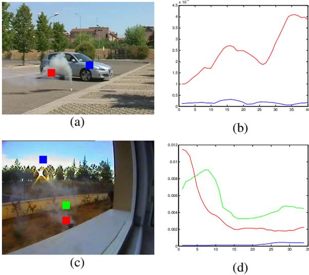
**Fig. 3.** (a)-(b) Variation of spatio-temporal energy for a block containing i) smoke (red block and line) and ii) a moving smoke colored object i.e. car (blue block and line), (c)-(d) variation of spatio-temporal energy for a block i) at the centre of smoke (red block and line), ii) at the edge of smoke (green block and line) iii) without smoke but with clouds (blue block and line).
