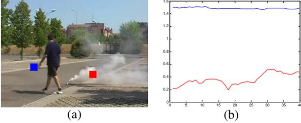
**Fig. 2.** Variation of spatial energy: i) a block with smoke (red block-line) ii) a block with a smoke colored moving object (blue block-line).
