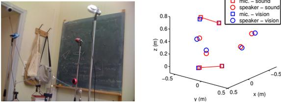
**Fig. 3:** Real microphone and speaker calibration setup, Left: the setup of microphones and speakers in an office, Right: the reconstructed sensor positions using TOA measurements (red) aligned with the positions estimated based on computer vision (blue).
