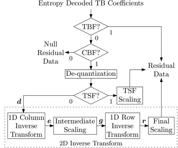
Fig. 1. Processing flow of the HEVC residual data decoding.
