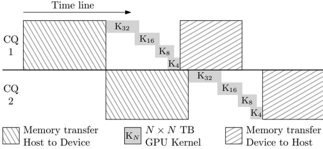
**Fig. 3.** Overlap of memory transfers and GPU kernels when using two OpenCL command queues (CQ).
