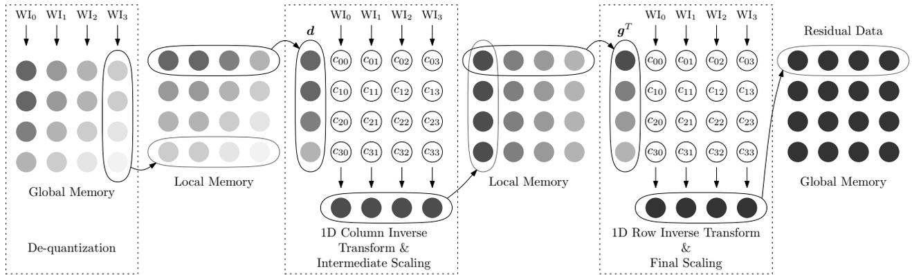
Fig. 2. De-quantization and 2D inverse transform implementation in the GPU for one  $4 \times 4$  TB processed by 4 work-items (WI).
