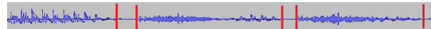
Fig. 1. Example of how to obtain borders between silence and phonemes, and vice versa.
