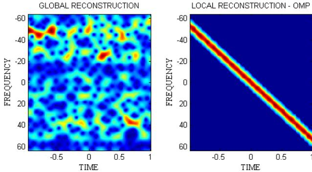
**Fig. 3.** Global and local reconstruction of chirp signal when 50% of data is missing
