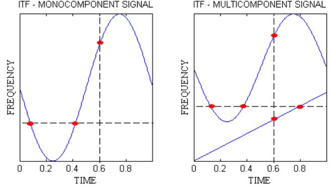
Fig. 1. Ideal time-frequency representation for given mono-component and multi-component signals.
