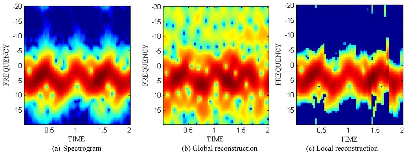
**Fig. 6.** (a) Spectrogram obtained from data with no missing samples; (b) Global reconstruction; (c) Local reconstruction of human gait signal when 45% of data is missing.
