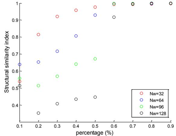
**Fig. 5.** Structural similarity index for the results using different window widths  $N_w$  and different percentage of present samples.
