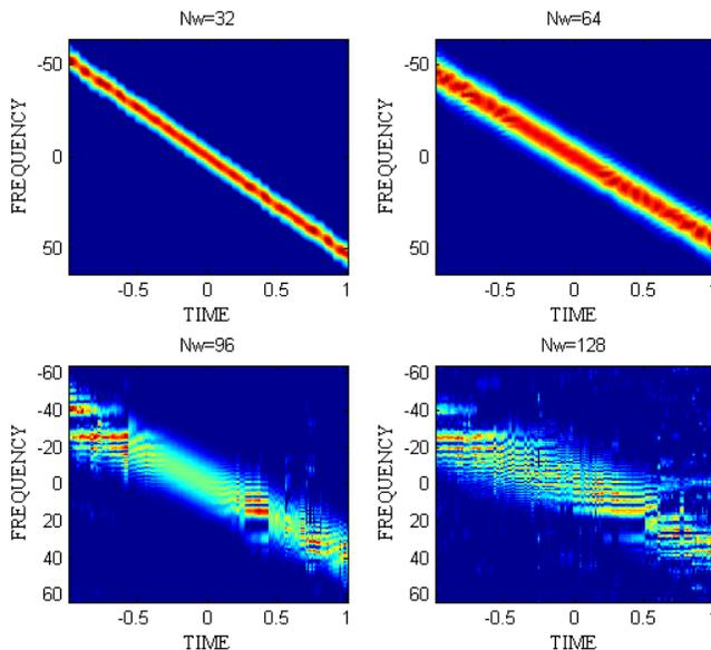
**Fig. 4.** Local reconstruction of chirp signal for different window widths:  $N_w=32$ ,  $N_w=64$ ,  $N_w=96$ ,  $N_w=128$ . 50% of data is missing.
