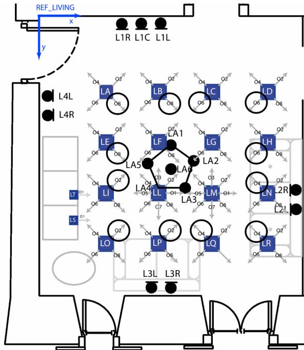
**Fig. 2.** Living room of the ITEA apartment of Fondazione Bruno Kessler (FBK) with the microphone array at the center and the 12 speaker positions employed in this work [provided by FBK].
