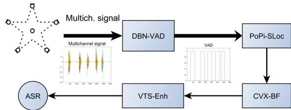
**Fig. 1.** Block diagram of the proposed system for distant speech recognition which consists of a 6-element microphone array, a voice activity detector based on deep belief networks (DBN-VAD), a speaker localizer based on the position and pitch plane (PoPi-SLoc), a convex-optimized beamformer (CVX-BF), a vector Taylor series enhancement (VTS-Enh) and an automatic speech recognizer (ASR).
