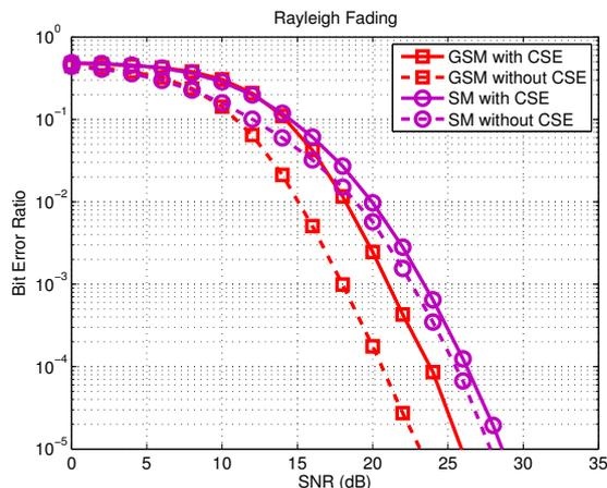
**Fig. 3.** ABER versus the SNR for GSM and SM over correlated Rayleigh fading channels for  $\eta = 12$ , and  $N_t = 128$ .
