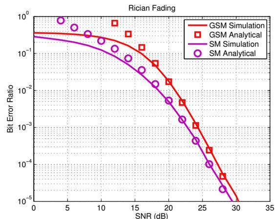
Fig. 2. ABER versus the SNR for GSM and SM over correlated Rician fading channels with  $K = 5$  dB for  $\eta = 8$ , and  $N_t = 16$ .
