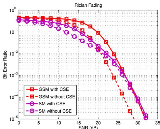
**Fig. 4.** ABER versus the SNR for GSM and SM over correlated Rician fading channels with  $K = 5$  dB for  $\eta = 12$ , and  $N_t = 128$ .
