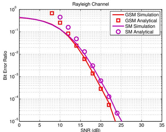
Fig. 1. ABER versus the SNR for GSM and SM over correlated Rayleigh fading channels for  $\eta = 8$ , and  $N_t = 16$ .
