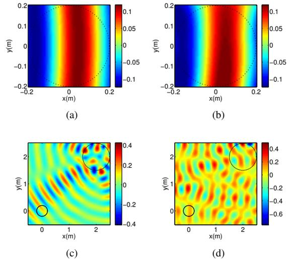
**Fig. 2.** For a desired line source at  $\mathbf{R}_0 = (-3, 0)$  m and  $f = 800$  Hz, the (a) desired and (b) reproduced soundfields over  $\eta$  and the (c) transmitted (without reflections) and (d) reproduced soundfields over  $\zeta$  and  $\eta$ .
