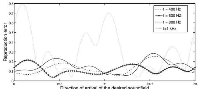
**Fig. 3.** Reproduction error (11) against DOA of the desired soundfield ( $\phi_0$ ) for a source distance of  $\|\mathbf{R}_0\| = 3.6$  m over a set of frequencies  $f = 400, 600, 800$  and  $1000$  Hz.
