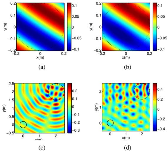
**Fig. 1.** For a desired line source at  $\mathbf{R}_0 = (2, 3)$  m and  $f = 800$  Hz, the (a) desired and (b) reproduced soundfields over  $\eta$  and the (c) transmitted (without reflections) and (d) reproduced soundfields over  $\zeta$  and  $\eta$ .
